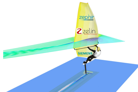
Fig. 2. 3D visualization of the current lines (in air and water)
